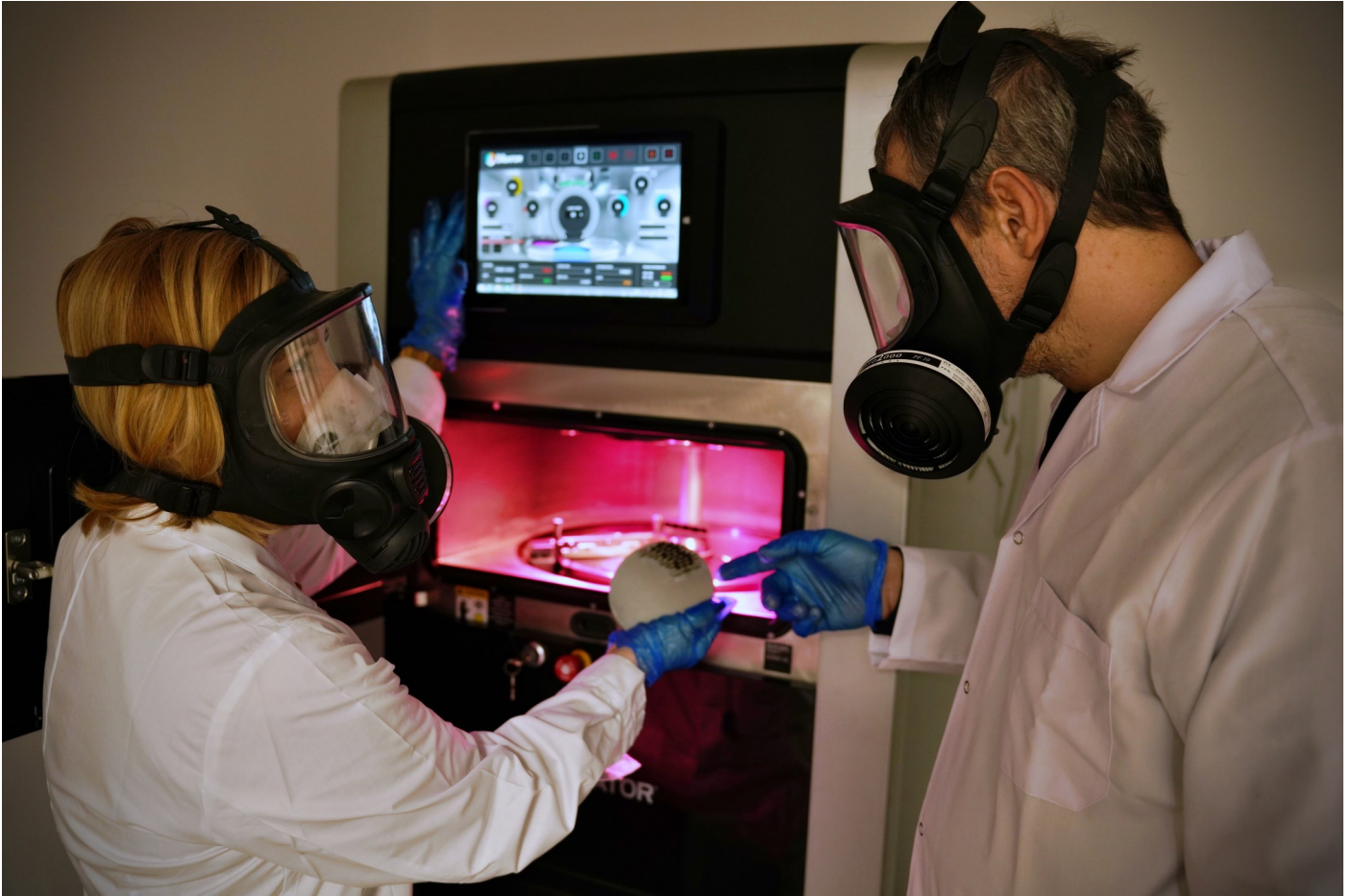
3D printed metal prototypes utilizing a Selective Laser Melting printer at the Additive Manufacturing Unit of CERTH|ITI.
